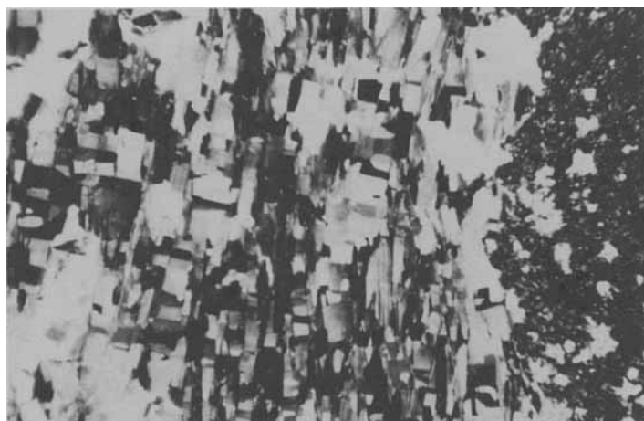
PLATE 6 Smectic G phase. Broken focal conic fan and mosaic textures. The fans have a characteristic patchwork or chequerboard appearance.
